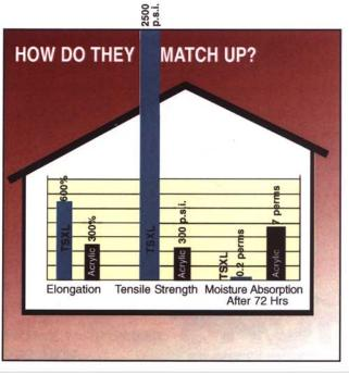
Water-based coatings should be used on breathing porous substrates such as stucco, block, interior concrete walls and certain polyurethane foam roofs. Solvent-based coatings have an extremely low perm rating, and act as a vapor barrier. Using a solvent based coating over these substrates is not recommended, as the product could trap moisture. This can cause blisters and delamination between the substrate and the coating.
